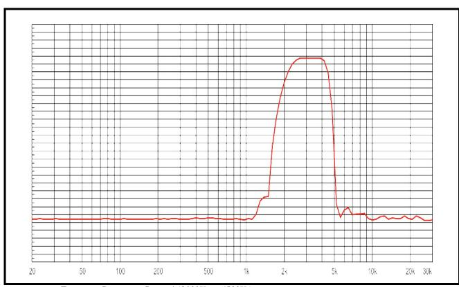
FIGURE 29. Frequency Response - Preset 4 (2100Hz to 4500Hz)
